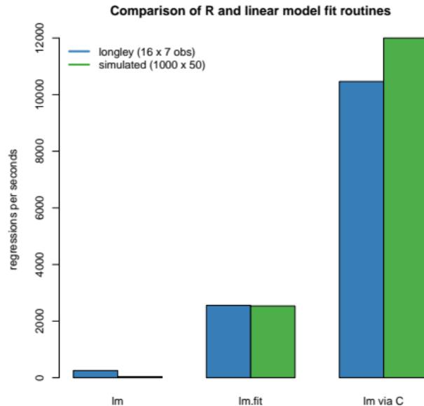
By inverting the times to see how many 'regressions per second' we can fit, the merits of the compiled code become clearer.
